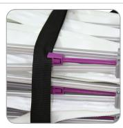
When packing unit in the bag, ensure that the strap is not partially wrapped around an arm. If it is, the arm will snap when pulled out of the bag.
